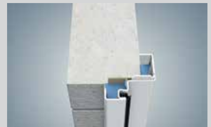
Montage in steen/beton
